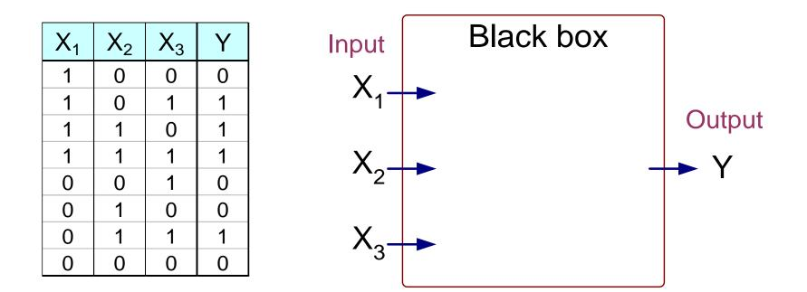
Output Y is 1 if at least two of the three inputs are equal to 1.
