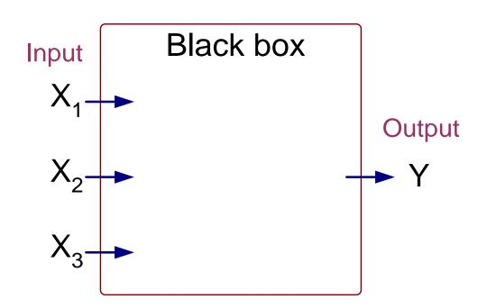
Output Y is 1 if at least two of the three inputs are equal to 1.
